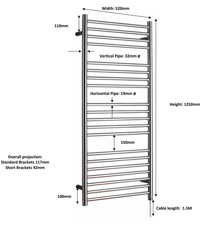
Constructed of 100% stainless steel Finish: Polished stainless steel Electric element: 240V 250W IP55 rated Built in thermostat rated at 60 degrees C Fitted with safety cut out fuse **CE Approved**
